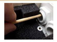
If the glands are inserted, push them out carefully from the inside of the box with a blunt rod of about 5 mm diameter at the side of the hole.
