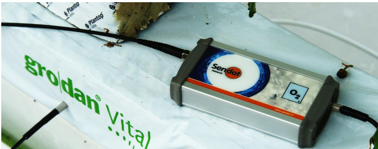
Figure 1: A Sendot O 2 sensor, probe inserted 1 cm above bottom substrate, in action.
